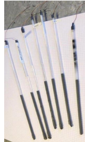
Figure 5. The JV-Elkem blackbody-based device. Left: indicated temperature of the sapphire rod blackbody thermometer during the copper freeze, showing data with and without optical-based corrections (the initial part of the freeze has been truncated). Right: Several instances of the device.
