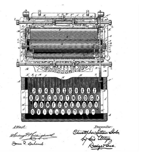
Figure 3: Diagram from Sholes patent US 568630
