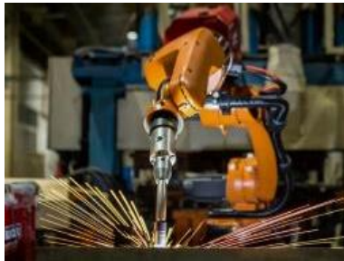
Automated Welding or Additive Manufacture (AM)
