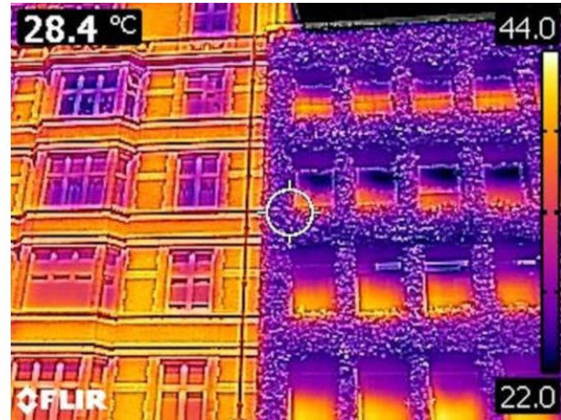
Figure 5-2 - Green wall vs conventional wall, Central London
