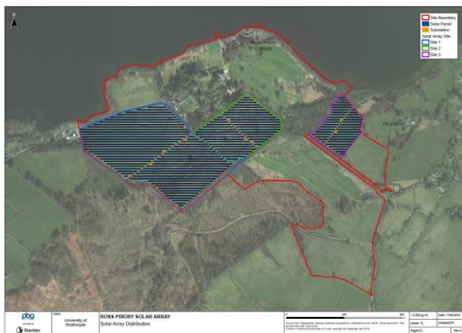
Proposal for a 21MW community solar array in partnership with Scottish Water at Ross Priory on 75 acres of rough grazing land. Taken from desktop study.
