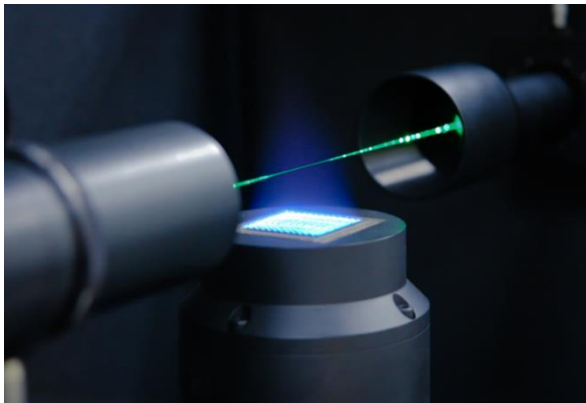
Figure 5. Left: Portable standard flame being interrogated by the laser Rayleigh scattering apparatus. Right: The gas metering and burner control system.
