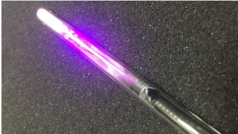
Figure 8. Fibre-optic ‘pig-tail’ phosphor thermometer. Excitation (blue light) yields phosphor emission (red light), giving a purple appearance.
