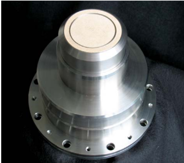
Burner with sintered bronze matrix (McKenna type)
