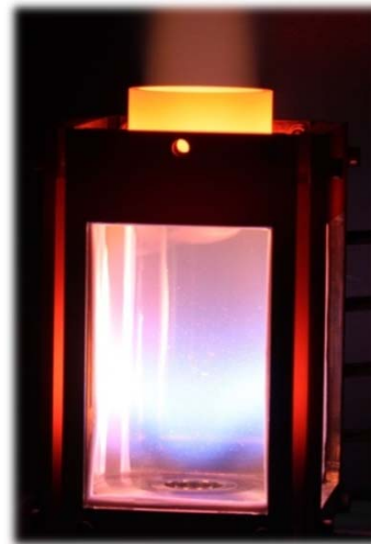
combustion chamber with quartz windows
