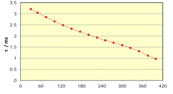
The phosphor **Mg<sub>4</sub>FGeO<sub>6</sub>:Mn** was calibrated by contact on the hot plate surface in the temperature range from 30 °C to 400 °C
