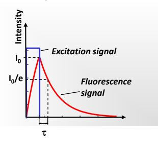
The surface temperature can be determined by measuring the fluorescence decay time, τ, of a temperature-sensitive phosphor layer coated on the surface under test
