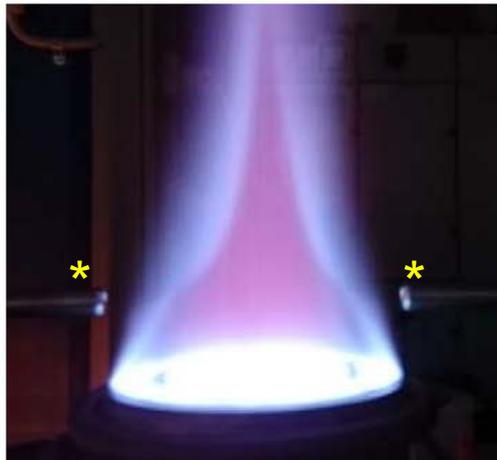
Flat flame burner: UV absorption path shown, gas path covered for reference measurements.
