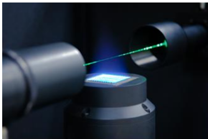
Figure 5: The NPL standard flame in the process of being interrogated using Laser Rayleigh Scattering. Photograph courtesy of NPL.
