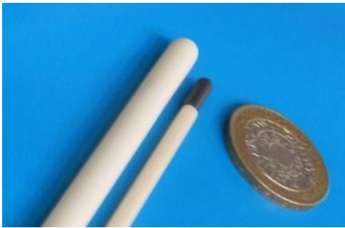
Melting and freezing of miniature FP crucible (Pt-Rh thermocouple, all in 7 mm o.d. sheath)
