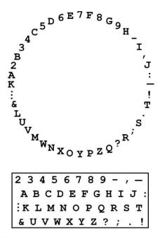
Figure 2: Sholes keyboard and typebasket with ABCDEF format
