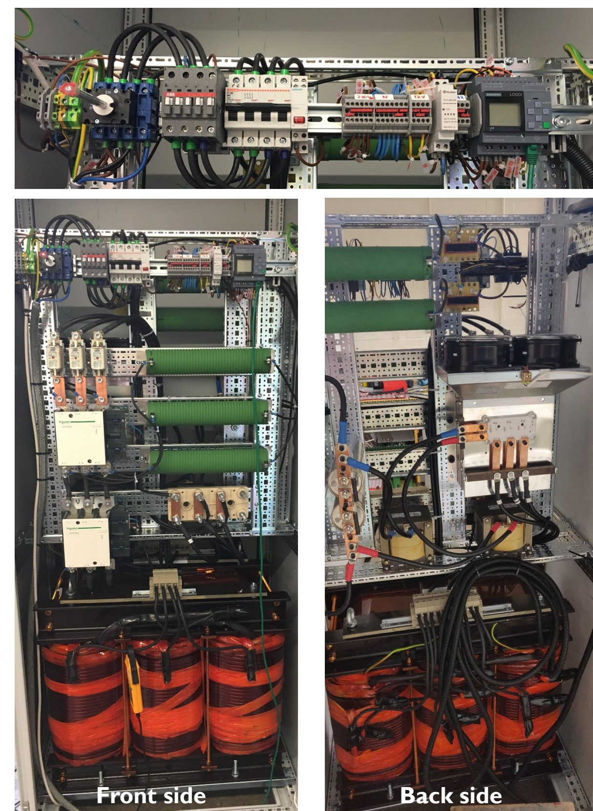
Figure 7. 90 kVA Rectifier converter. Built with Z. Blatsi
