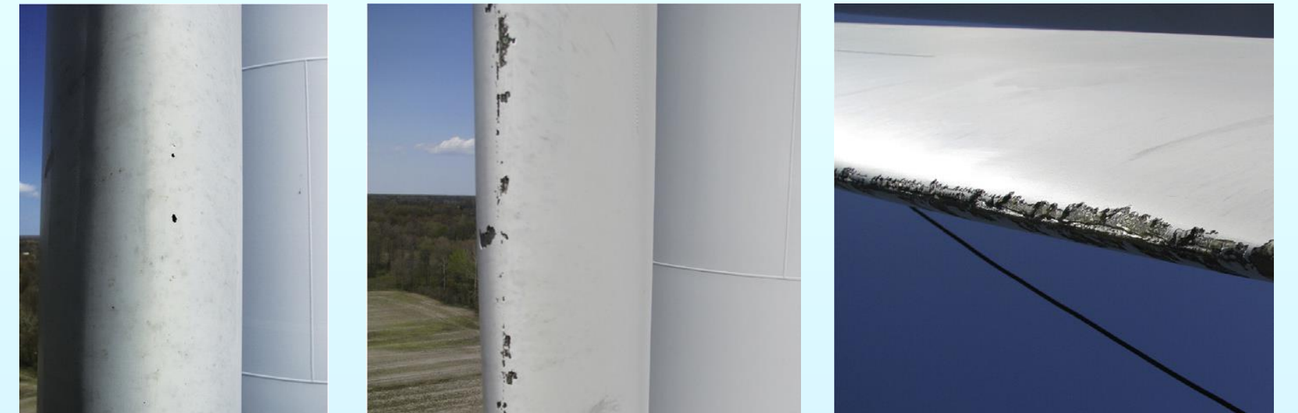
Images: H. M. Slot, E. R. Gellinck, C. Rentrop, and E. Van der Heide, "Leading edge erosion of coated wind turbine blades: Review of coating life models," Renewable Energy
