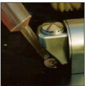
Effortlessly determine the amount of minor components in your liquids with the TumbIIR sampling system of the Agilent 4500t FTIR
