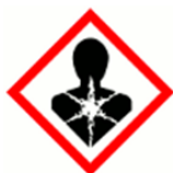
Serious health hazard (Symbol: health hazard)
