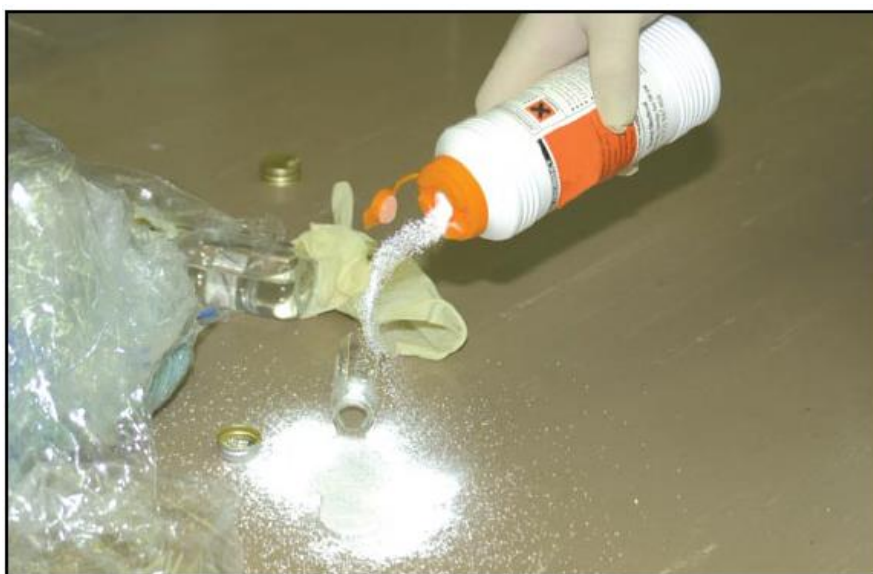
Figure 1. Dealing with a small volume liquid spill. (Image: ACDP Guidance on The Management and Operation of Microbiological Containment Laboratories).
